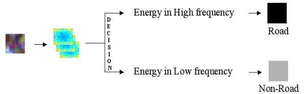
Figure 2: Decision criterion for the MESE edge detection technique for multispectral images
