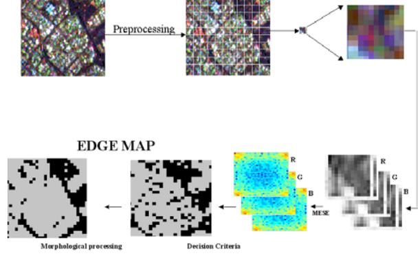
Figure 1: Flow chart for the MESE edge detection technique for multispectral images
