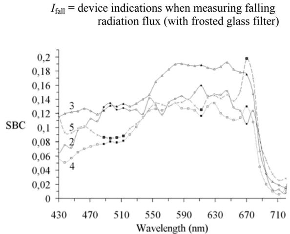
Figure 2. SBC Spectral distribution recorded at 45° in four points
