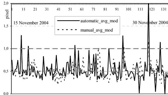
Figure 4. Average module of GCP discrepancies of automatic and manual navigation procedures.
