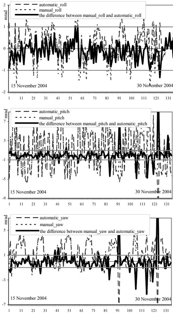
Figure 3. Comparison of roll, pitch and yaw estimations calculated automatically and manually for time interval November 15-30, 2004. 1 mrad is equivalent of 1 pixel accuracy.
