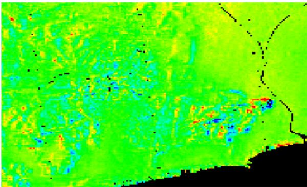
*Figure 7. DEM error from JERS-1 SAR winter pair 03Dec1995 -16Jan1996. Baseline is 606 meters.*
