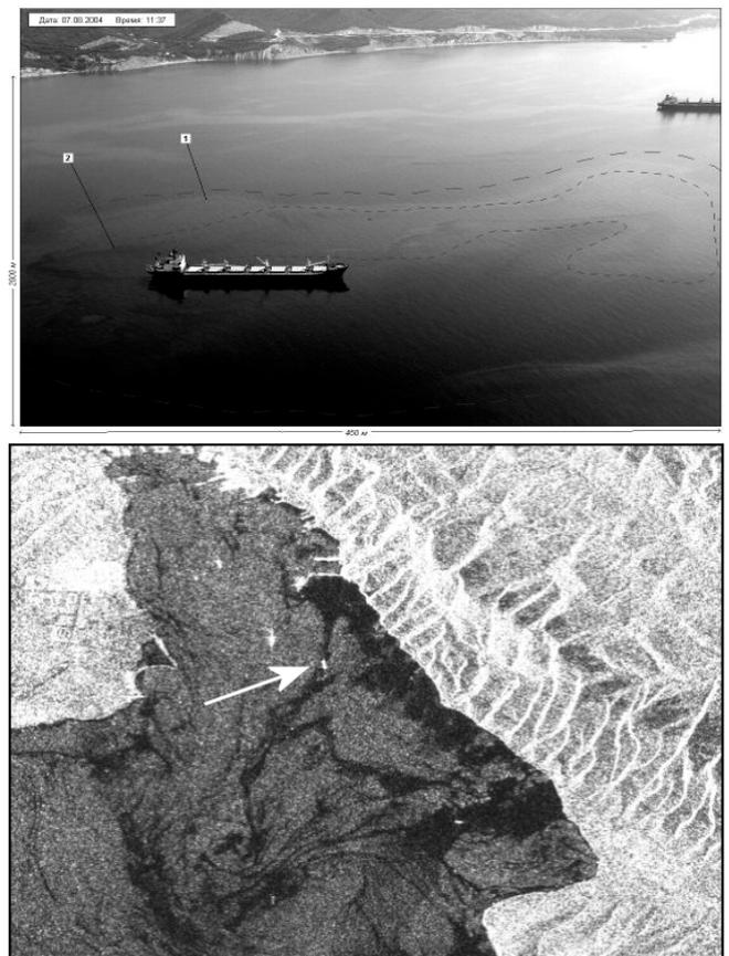
Figure 2. The Georgios III oil spill on 7 August 2004. Top: aerial photograph of the spill. Bottom: Envisat ASAR image of oil in Tsemesskaya Bay 12 hours later. Arrow shows the tanker position.
