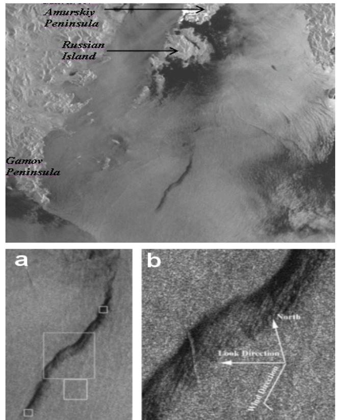
Figure 4. ERS-2 SAR image from 22 September 1997 at 02:00 UTC showing oil pollution in Peter the Great Bay, Japan Sea. Below this (a) shows an enlarged fragment of oil spill (large white rectangle) used for estimating the wind direction (b).
