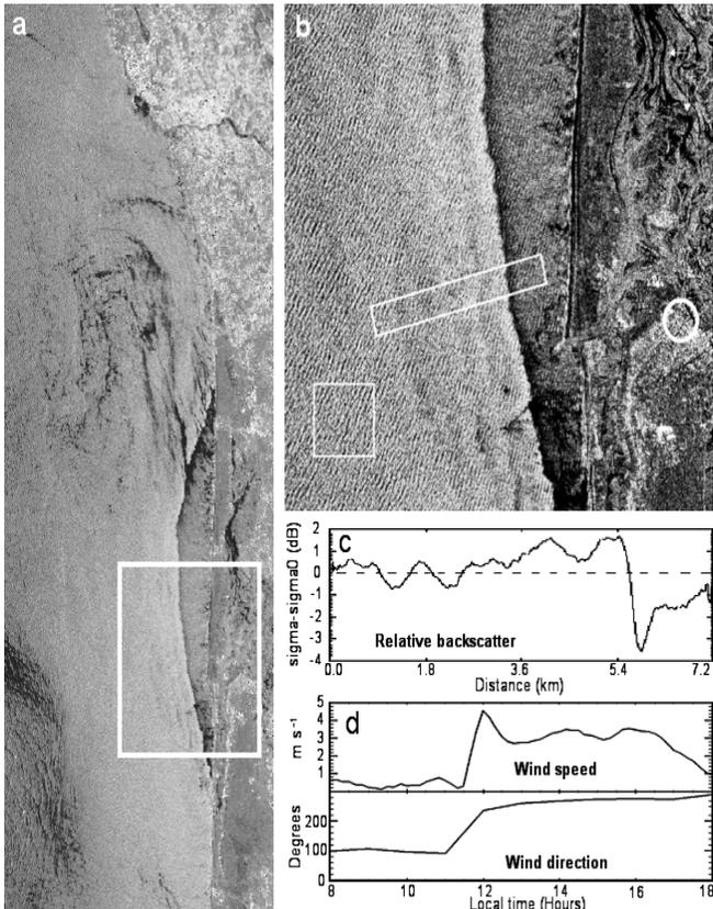
Figure 5. Oil look-alike caused by atmospheric internal waves. a) ERS-2 SAR scene from the west coast of Portugal on 26 September 2001 at 11:19:57 UTC. b) Extract from the image showing wavelike features. c) Relative backscatter profile obtained from the area of the long rectangle in b. d) Wind speed and direction recorded at the meteorological station near Aveiro indicated by a circle in b.
