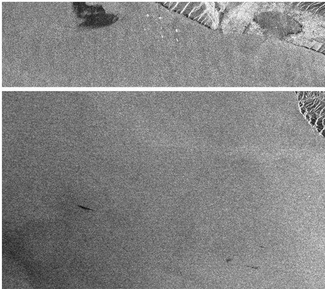
Figure 1. Examples of minor oil spills. ERS-2 SAR from 20 August 2004 (top) shows a dark patch representing waste water discharge on the anchorage site near Cape Doob. Below: Envisat ASAR data from 23 Aug. 2004 show pollution 65 km offshore.
