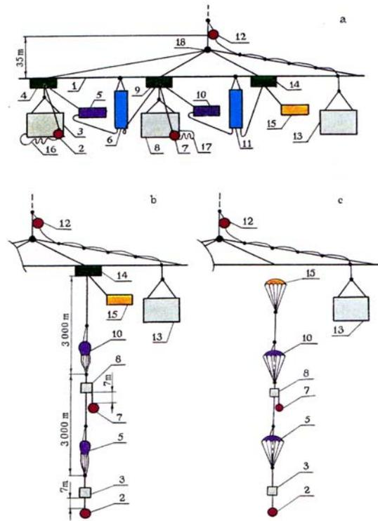
Figure 1. Scheme of balloon magnetic gradiometer in the starting (a), working (b) positions and at the finish stage (c) of flight
