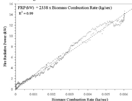
**Figure 1: Experimentally determined relationship between FRP and combustion rate**
