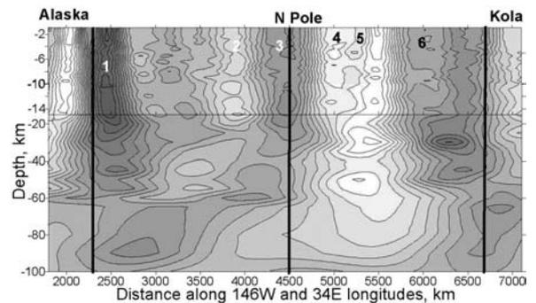
Figure 3. Vertical cross-section of the deep structure along the geotraverse in Fig. 2. Numbers of the bodies correspond to Fig. 2. Boundary of the asthenosphere is on depth 60 km. Height exaggeration is different for layer up to 15 km and for layer 15-100 km.
