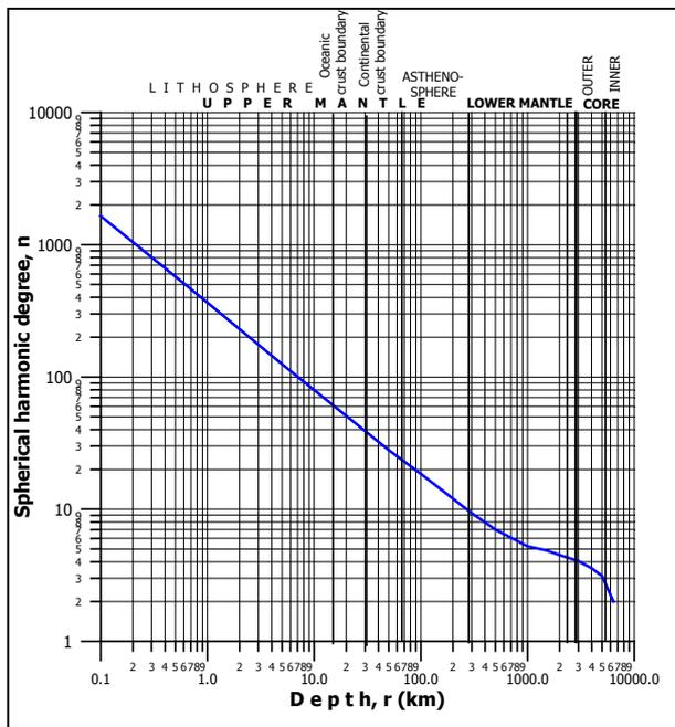
Figure 1. Relationship between harmonic degrees  $n$  and depths  $l$  disturbing layers of the Earth. Value  $n$  is a sum of harmonics in a range from degree 2 up to  $n$ . Depth  $l$  corresponds to upper cover of the disturbing layer; its thickness is considered from the center of the Earth.
