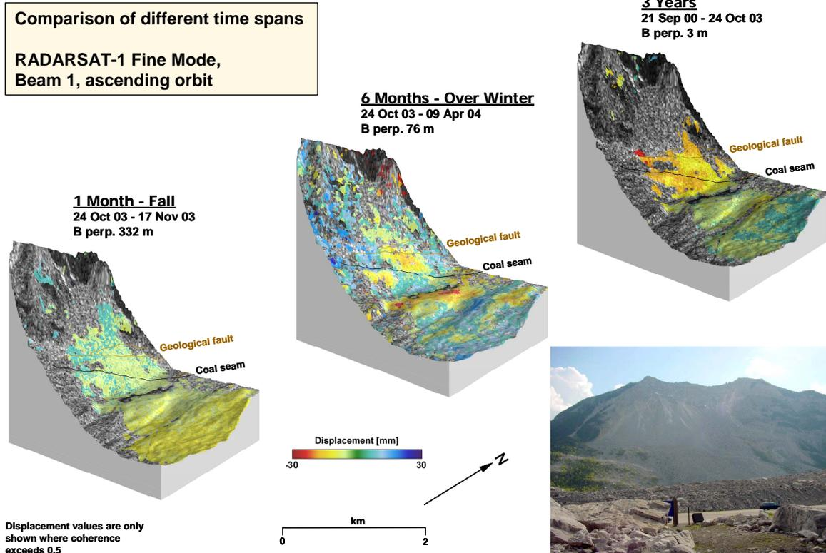
Figure 1. RADARSAT-1 InSAR displacement maps for three different time spans between 2000 and 2004.
