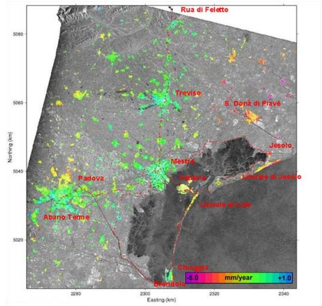
Figure 4. INSAR land subsidence map (in mm/year) of the Lagoon of Venice for the time period 1993-2000 with ground based levelling network superimposed
