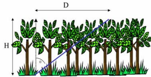
Figure 3. Schematic representation of the acquisition distance at a given zenith angle  $\theta$ . The distance  $D$ , where a gap can be measured at the top of the canopy, is equal to  $\tan(\theta) * H$ .
