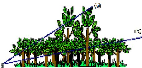
Figure 6. Paths from different zenith angle through a canopy should go through the same amount of vegetation. When using a small number of segments, the chances of having different foliage density at different VZA are very large.
