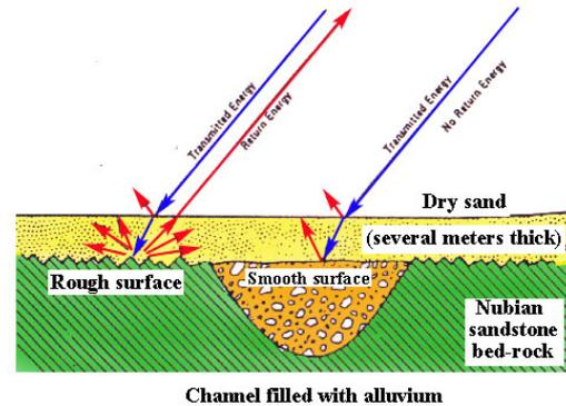
Figure 2. Radar detection of hidden water
