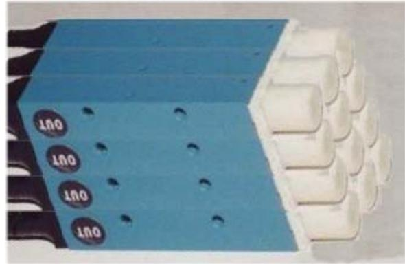
Figure 8. A prototype of FPA with MMIC receiver modules at 26-30 GHz.
