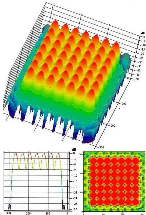
Figure 5. Three dimensional 7x7 beam pattern of 2 m Cassegrain antenna in 3 mm band (top), one dimensional cut (left bottom), isoclines (right bottom), the feed taper is -10 dB
