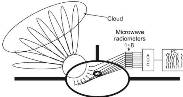
Figure 7. Cloud mapping with Luneberg lens and 8 radiometers
