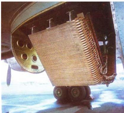
Figure 1. Scanning antenna system installed at airplane-laboratory ILT-18
