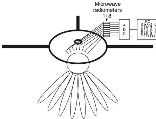
Figure 6. Luneberg lens and 8 radiometers
