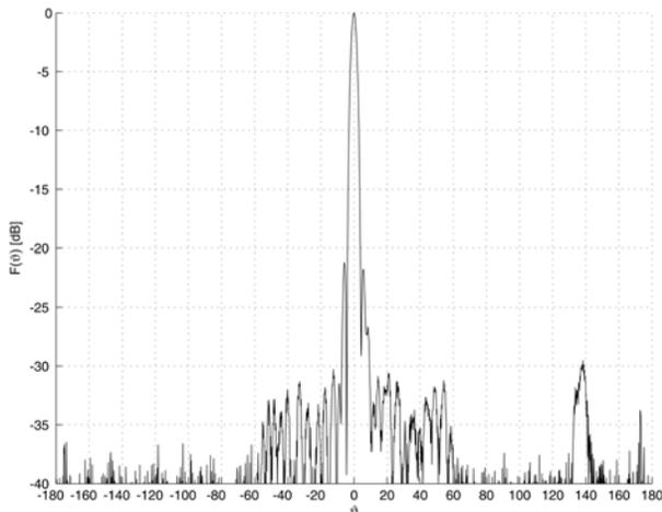
Fig.4. Radiation pattern of spherical Luneberg lens by Konkur Co. at f=10.79 GHz in E-plane
