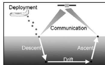
Figure 3. Deployment and mission design of THE ABYSS probes system (Ecosphere, 2003).
