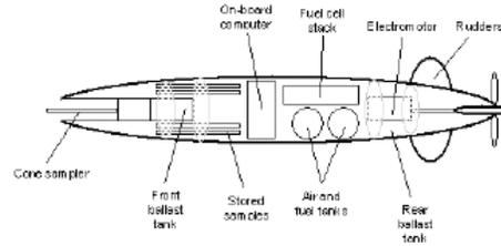
Figure 2. The proposed ocean core sampler (Ecosphere, 2003).
