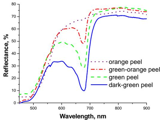
Figure 2. Reflectance spectra of orange peel samples for the cultivar Navel with different coloration of the peel.
