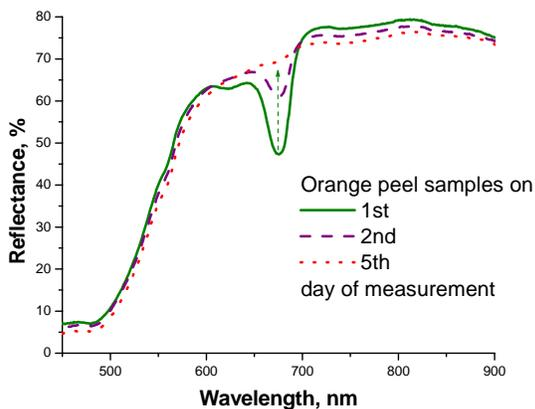
Figure 3. Reflectance spectra of orange peel samples for the cultivar Navel during storage at laboratory conditions (medium light and room temperature).
