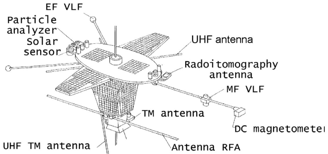
Fig.1. COMPASS microsatellite
