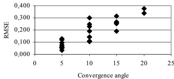
Figure 4. Relation between the convergence angle and the precision of the DSM expressed as RMSE in meters.
