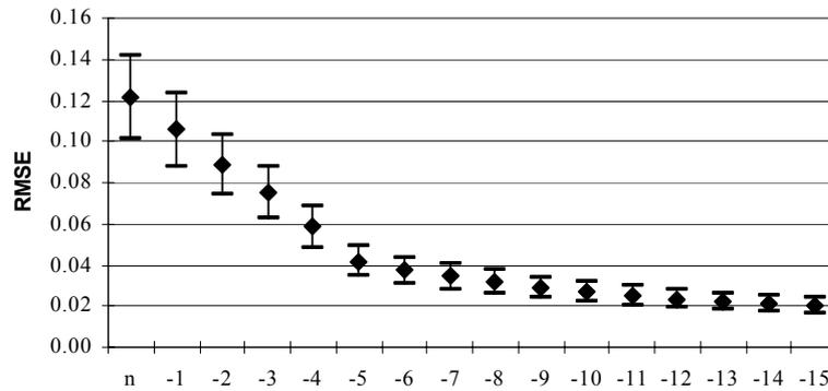
Figure 5. Improvement of the precision of the DSM with the elimination of the check points with the greater errors. The vertical strokes show the value of the confidence interval at the 95%.
