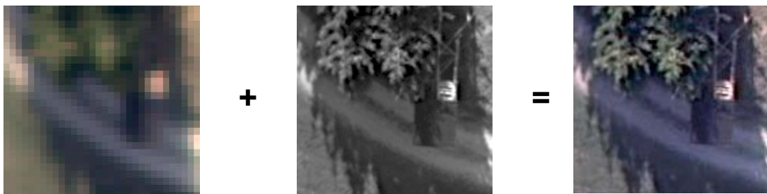
Fig.4: Example of a pan-sharpened image of a digital frame sensor
