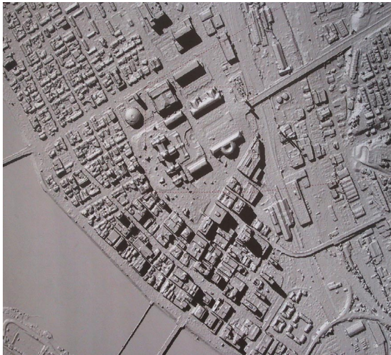
Fig.7: DSM derived from 30cm GSD ADS40 three line imagery
