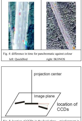
Fig. 5: location of CCDs in the focal plane – misalignment in the focal plane and vertical shift against the focal plane
