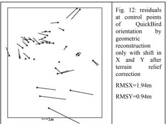
The exterior orientation can be used also for a verification of the calibration and a check of the quality of the direct sensor orientation. A QuickBird scene has
