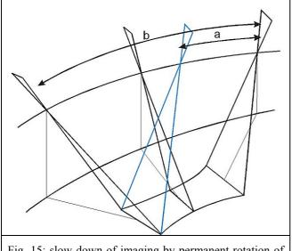
Fig. 15: slow down of imaging by permanent rotation of view direction slow down factor = b / a
