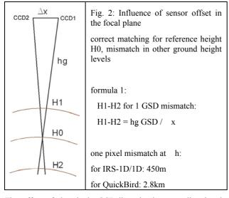
The offset of the single CCD-lines in the scan direction is causing a different view direction (figures 2 and 3). For a chosen reference ground height, the individual images can be matched without discrepancy, but if a scene has a stronger variation of the ground height, a mismatch may be caused. For example in the case of IRS-1C/1D the difference in the focal plane corresponds to 8.6km difference in the corresponding
