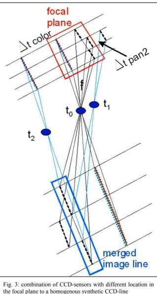
Only moving objects do show some effects. Because of the different imaging instant for colour and panchromatic in pansharpened images in the case of IKONOS the colour of fast moving cars is shown behind the grey value image and for QuickBird it is shown in front (figure 4). This effect can only be seen at fast moving objects; it is usually not disturbing and not affecting the objects important for mapping purposes.
