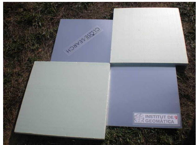
Figure 6: Thermal passive target used during the first test campaign in CLOSE-SEARCH
