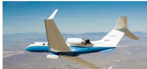
Figure 4. UAVSAR in pod carried by NASA G-III
