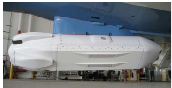
Figure 8. Pod carrying Ka-band antennas on lower surface.
