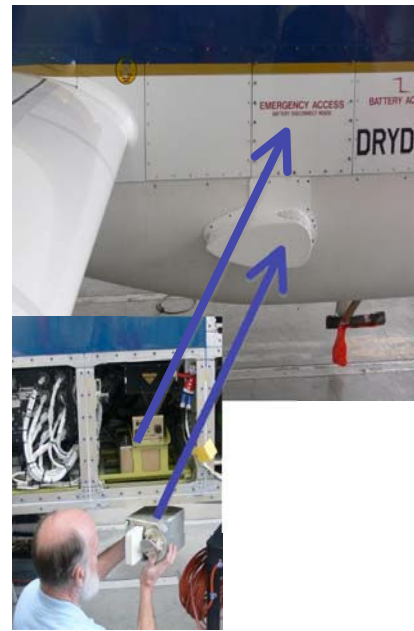
Figure 14. JPL Microwave Temperature Profiler located on the Global Hawk
