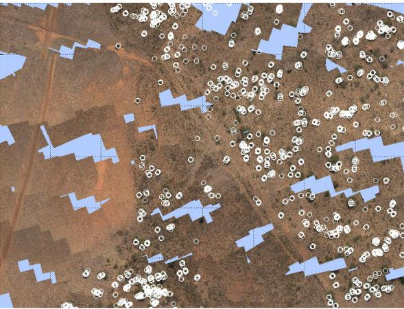
Figure 6: Detection results over a selected mission area, the white circles are the points of detection, multiple circles occasionally shows up for the same tree because the same tree crown was detected in separated frames. The individual image frames are joint together using algorithm described in (Bryson, 2010)
