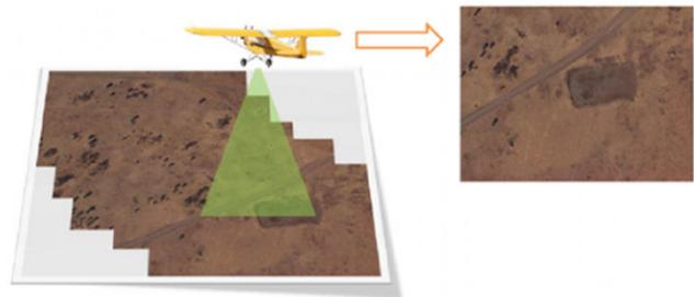
Figure 1. Scaled down J3 Cub: This platform is used to collect aerial image data over Julia Creek, Queensland, Australia. The mission area is flat with trees distributed sparsely, the data set is ideal to test the object detection algorithm.
