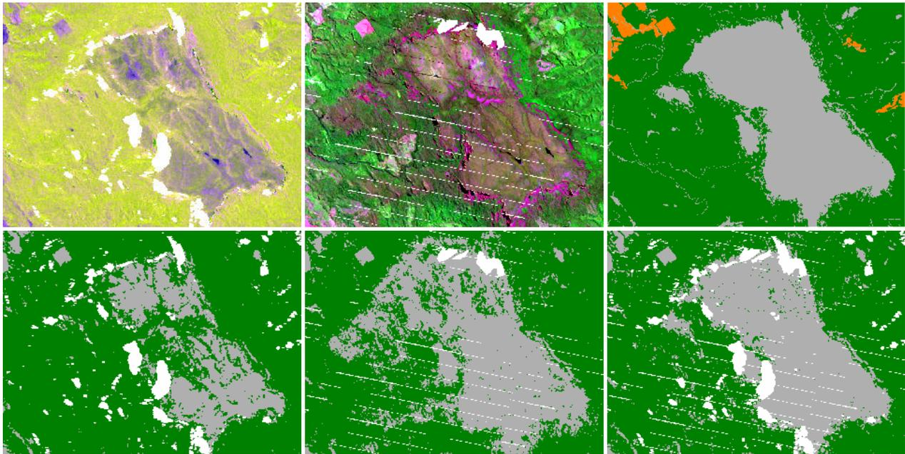
Figure 4. Example of MLC outputs for the Ben Lomond area (20km×15km). In all plots, white pixels indicate masked areas. *Top row, left*: PALSAR data (HH/HV/HH-HV in R/G/B). *Top row, middle*: Landsat data (bands 5/4/2 in R/G/B). *Top row, right*: TASVEG map with forest in green, non-forest in grey, and plantations in orange. *Bottom row, left to right*: maximum likelihood F/NF classifications with forest in green and non-forest in grey for PALSAR, Landsat, and combined PALSAR–Landsat data.
