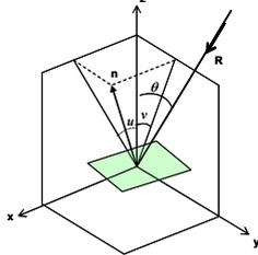
Figure 2. Surface tilt angles:  $u$  is the tilt angle in the range direction, and  $v$  the tilt angle in the azimuth direction.
