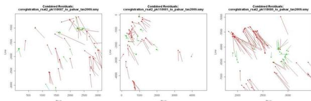
Figure 6. RMS Error displacements of co-registration of RADARSAT-2 and PALSAR images: NE (left), NW (middle) and SW (right) Tas.
