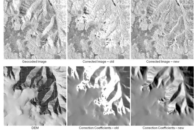
Figure 3. Comparison of terrain slope corrections by a method modified from C-correction for optical process and the new approach.
