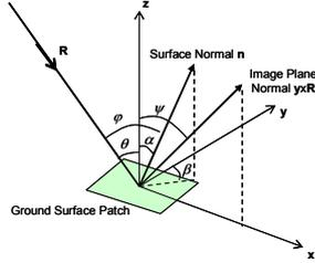
Figure 1. Scattering geometry of a tilted ground surface patch and its projection into the SAR image coordinates.
