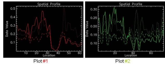
Figure 4. Spatial profiles of lines across terrain ridges for pre-correction (solid line), correction by C-correction (dotted line) and the new approach (dash-dot line).
