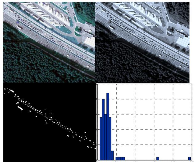
Figure 6. Aerial multispectral photo (top left) on Munich-Salzburg highway with 3K Camera (courtesy DLR). With a multiplayer feed-forward network cars on the highway can be extracted and classified by size (bottom right)
