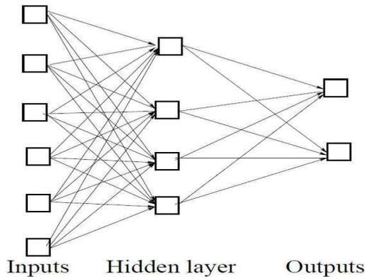
Figure 2. Schematic diagram of typical a multilayer feed-forward network.
