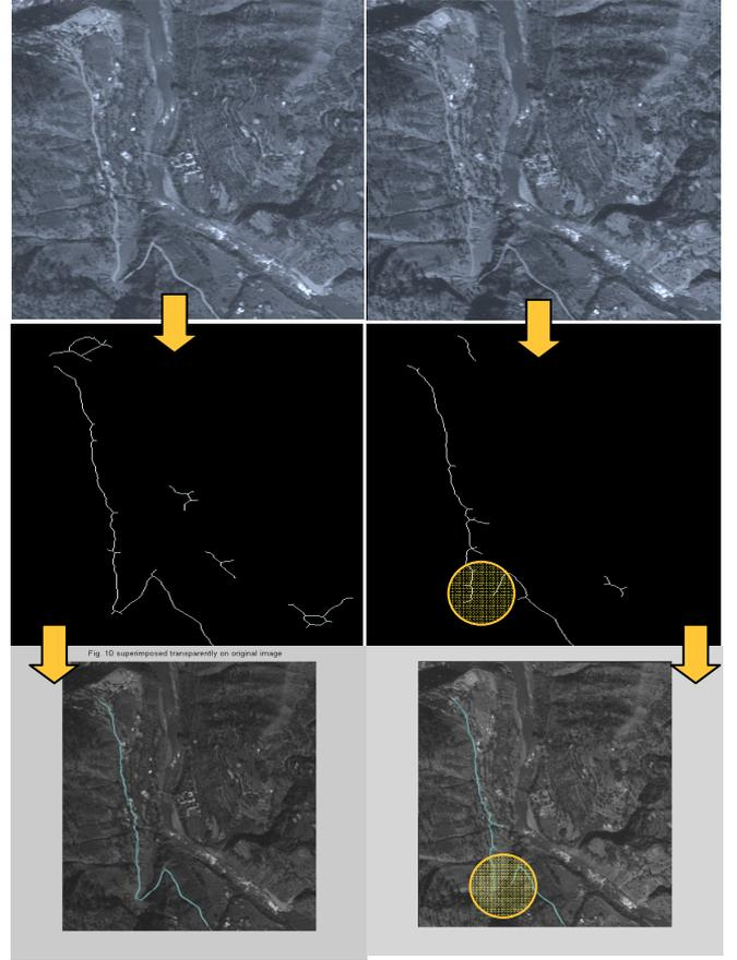
Figure 1. Automatic procedure to search the roads present on the SPOT 5 images (5 m resolution). The technique was applied before (above) and after (below) the earthquake that struck the Kashmir region on October 2006. This technique allowed to find the damages on the infrastructures.
