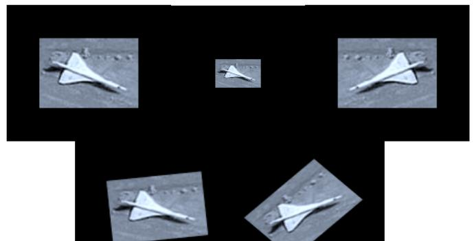
Figure 4. Concorde used as sample in order to extract it by Geometrical Moment Invariant. The shape signature of this object is always the same regardless of the applied rotations (below), scale factor (above) or translations.
