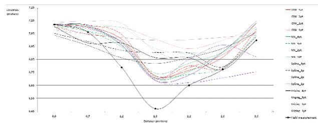
Figure 2. Comparison between DTMs derived from LiDAR data and field measurements on a ditch
