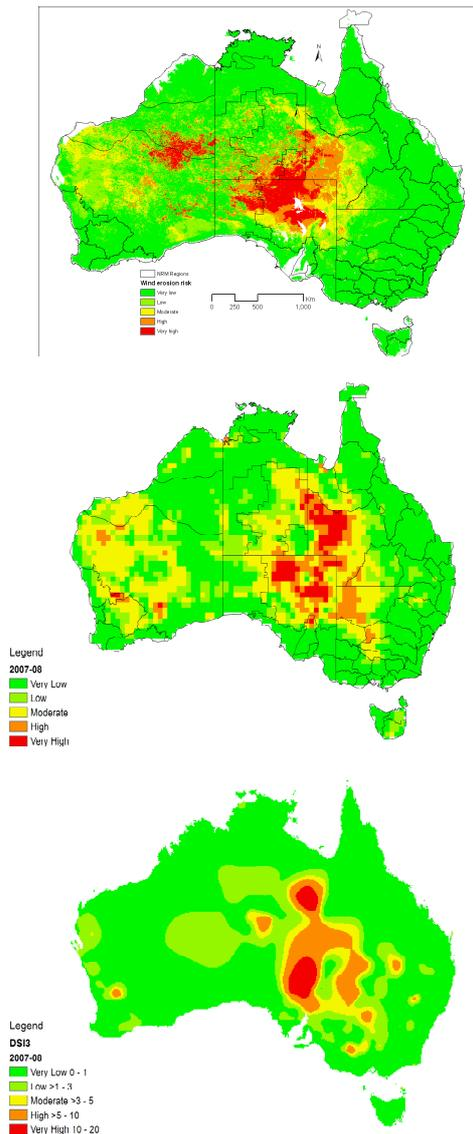
Figure 7. Comparison of modelled wind erosion risk with CEMSYS and dust storm frequency in 2007-08. Top: wind erosion risk estimated using the rule-set approach (this study); Middle: CEMSYS modelled dust concentration; Bottom: Estimated frequency of dust-storms over Australia (Middleton, 1984)
