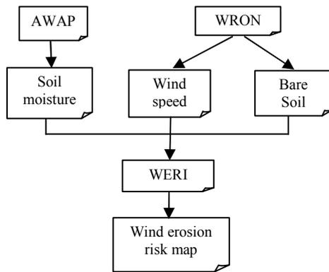
Figure 1. Procedures for calculating Wind Erosion Risk Index (WERI) from time-series Australian Water Availability Project (AWAP) and Water Resource Observation Network (WRON) products.
