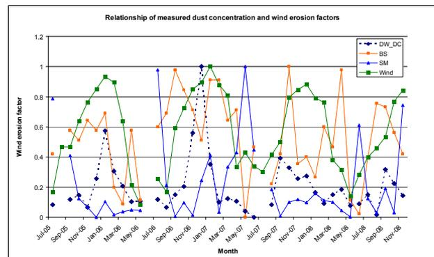
Figure 2. Relationship of measured dust concentration (at the DustWatch nodes) and the wind erosion factors.
