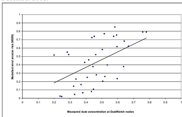
Figure 10. Relationship and trendline between modelled wind erosion risk (WERI) and measured dust concentration from DustWatch nodes. Values are rescaled to the same range (0-1) and extreme values at both ends were removed.
