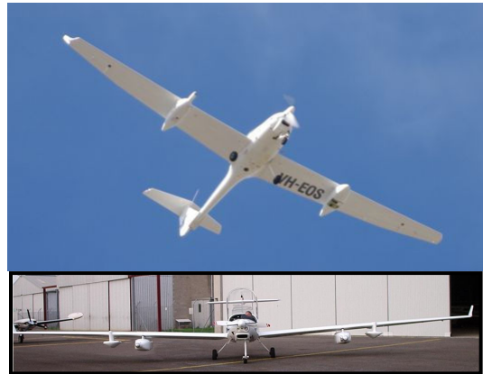
Figure 1: Top: One of ARA's ECO-Dimonas showing the two underwing pods carrying a lidar, a hyperspectral scanner, and aerial camera and some other sensors. Bottom: ECO-Dimona showing the four-pod configuration.
