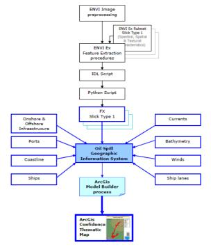
Figure 3. Workflow of automatic oil spill system approach.
