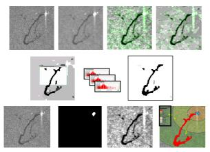
Figure 6. Sequence of steps needed to extract the oil slick from the original SAR image (top and middle) by using ENVI Ex and exporting its results in GIS environment for using contextual information (bottom).
