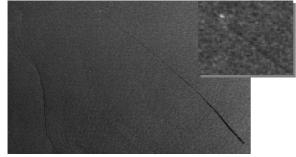
Figure 2. ENVISAT ASAR WSM. Mediterranean Sea. Ship is clearly visible as bright white spot. While two slicks were detected the right one is correlated with a ship.
