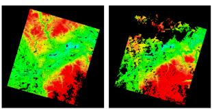
Figure 2. Cartosat-derived DEMs from 05.03.2009 (left) and 19.09.2010 (right). No correlation areas are coloured in black.
