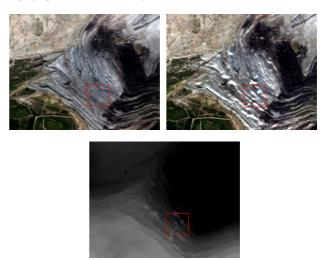
Figure 4. Effect of DEM errors on illumination correction. Atsensor radiance image (top left) with shadows. Overcorrection plus artefacts in surface reflectance image (top right) caused by DEM errors in slopes of mining area (bottom).
