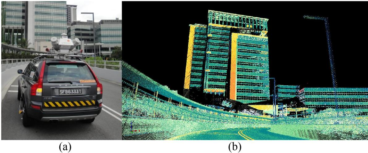
Figure 8. (a) Mobile Mapping System and (b) point cloud example data at CREATE building at NUS campus “University Town”
