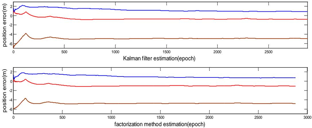
Figure4.2 kinematic positioning results for Kalman filter and factorization
