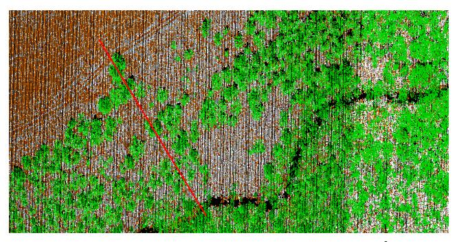
**Figure 1.** Example of airborne LIDAR data, density is about 4 points/m<sup>2</sup>. Red line is the axis of profile (see Fig. 2, below)
