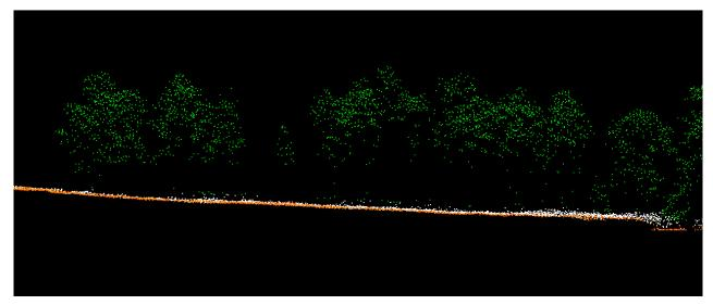
**Figure 2.** Profile along the red line through the LIDAR data. Green points – the upper parts of canopies, yellow and white – the surface of the relief – even under the canopies.
