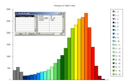
**Figure 4.** Histogram of distribution of the single trees according to their heights within previously mapped contour of the forest, defined by the experts as "homogenious". Done using 4 point/m<sup>2</sup> airborne laser scanning.
