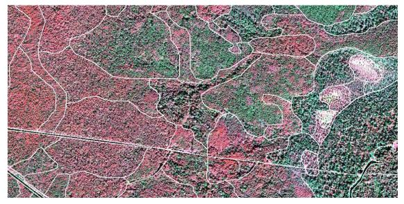
**Figure 5.** Example of usage WorldView2 infrared data for correction of zonal borders during forest inventorying according to the type of forest. This data is to be used later (together with the airborne LIDAR data) to renew statistics.
