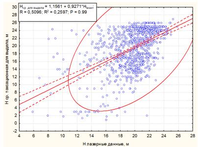
**Figure 6.** Dependency between mean heights of the trees, defined manually in the field (Y axis) and using the LIDAR data (X axis). Diagram belt using 978 semi-homogeneous regions.
