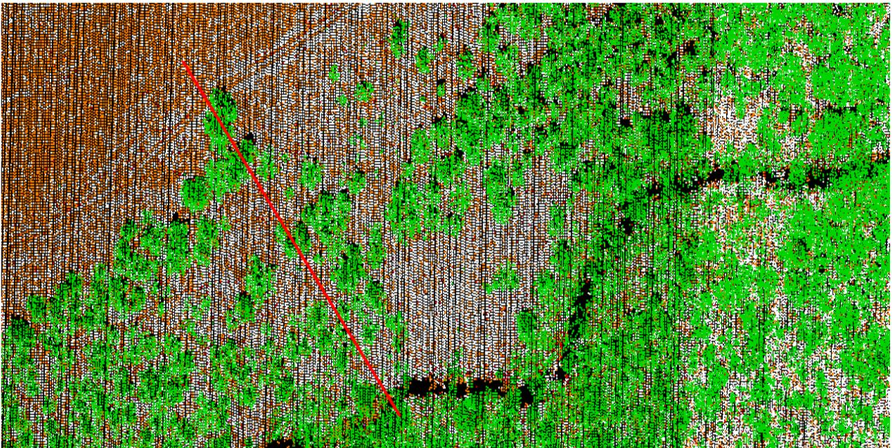
**Figure 1.** Example of airborne LIDAR data, density is about 4 points/m<sup>2</sup>.
