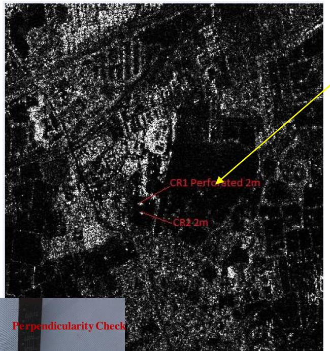
Response of perforated CR in L-band airborne image of 14<sup>th</sup> February 2018
