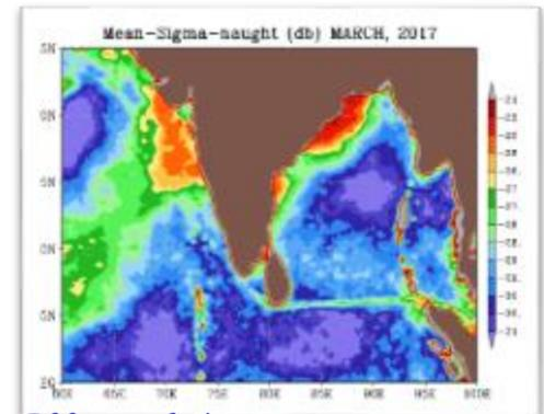
Effect of ships on scatterometer measurements
