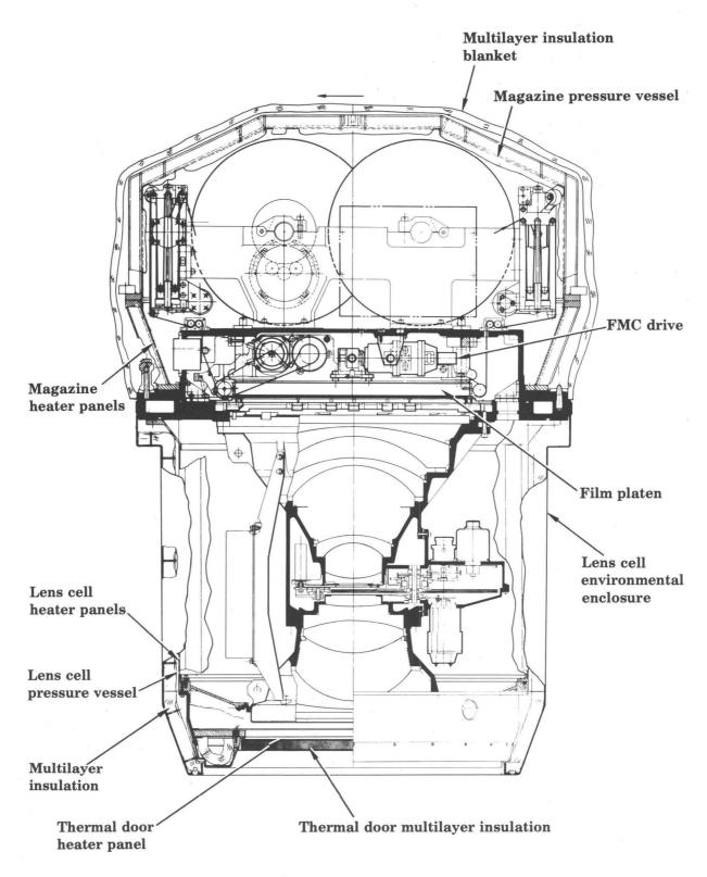
Fig. 1 - LFC internal environment control facilities
