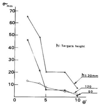
Fig. 9 Relation between  $\theta$  and Standard deviation  $\sigma_z$  in z-direction
