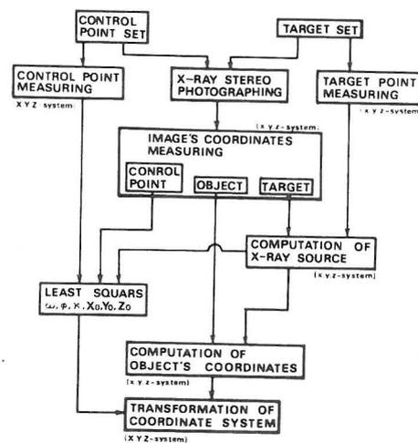
Fig 1-b Fundamental flow chart
