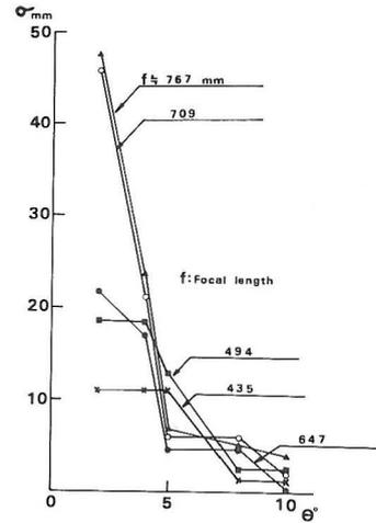
Fig. 10 Relation between  $\theta$  and Standard deviation  $\sigma_z$  in z-direction
