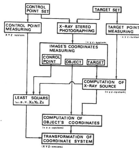
Fig 1-b Fundamental flow chart
