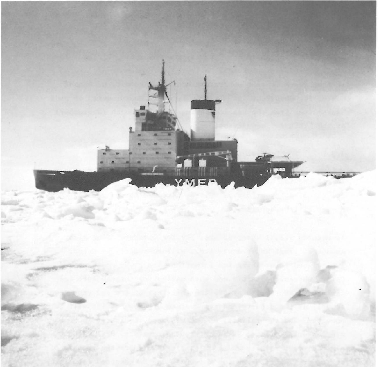
Fig. 2. The Swedish icebreaker YMER breaking her way in hummocked ice in the Bay of Bothnia. Displacement 8,000 tons, length over all, breadth and draught about 105 x 24 x 7.3 m; D/E machinery output 22,000 shp, 4 propellers, 2 fore and 2 aft, speed 19 kn. Designed in close cooperation between the Swedish and Finnish Administrations of Shipping and Navigation; Builders WÄRTSILÄ HELSINKI SHIPYARD.
