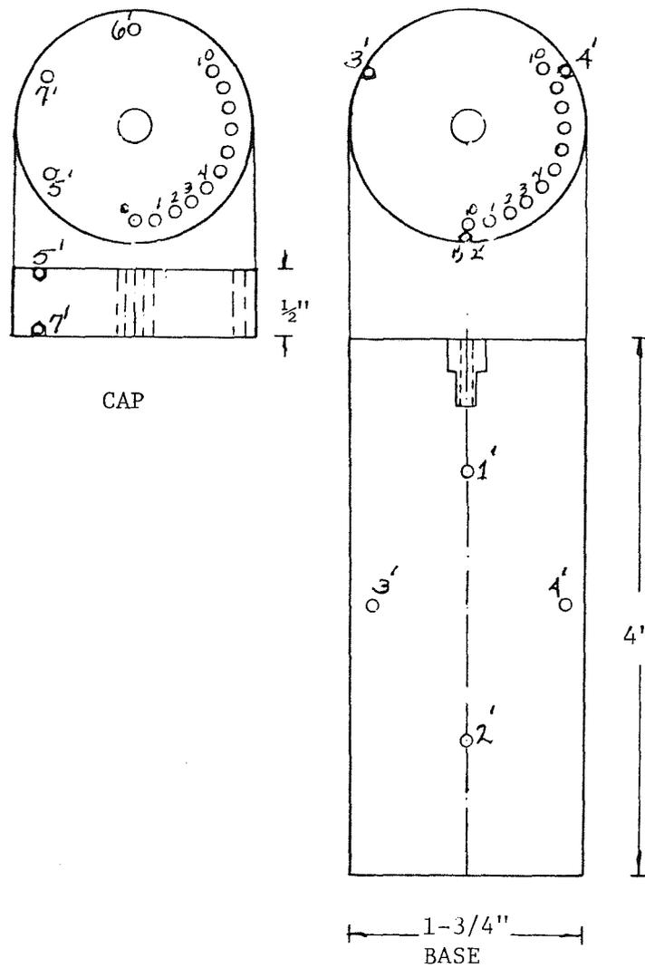
Figure 3. Plastic model used to compare Seattle and Cleveland Photogrammetry Systems.
