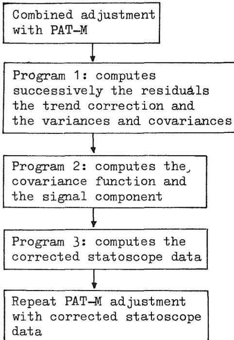
Fig. 1: Initial procedure
