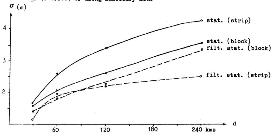
Fig. 5. Effect of using filtered statoscope data
