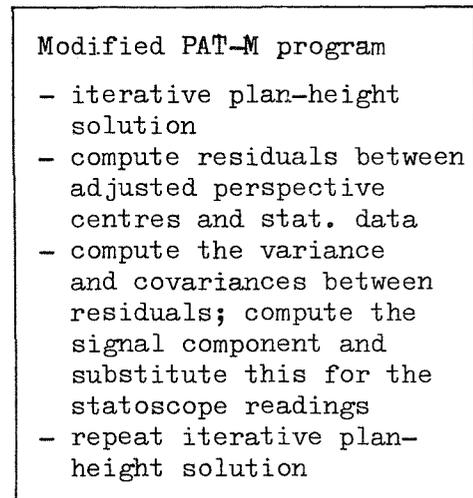
Fig. 2: Modified procedure
