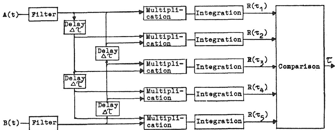
Fig.3: Establishing parallax from maximum correlation function
