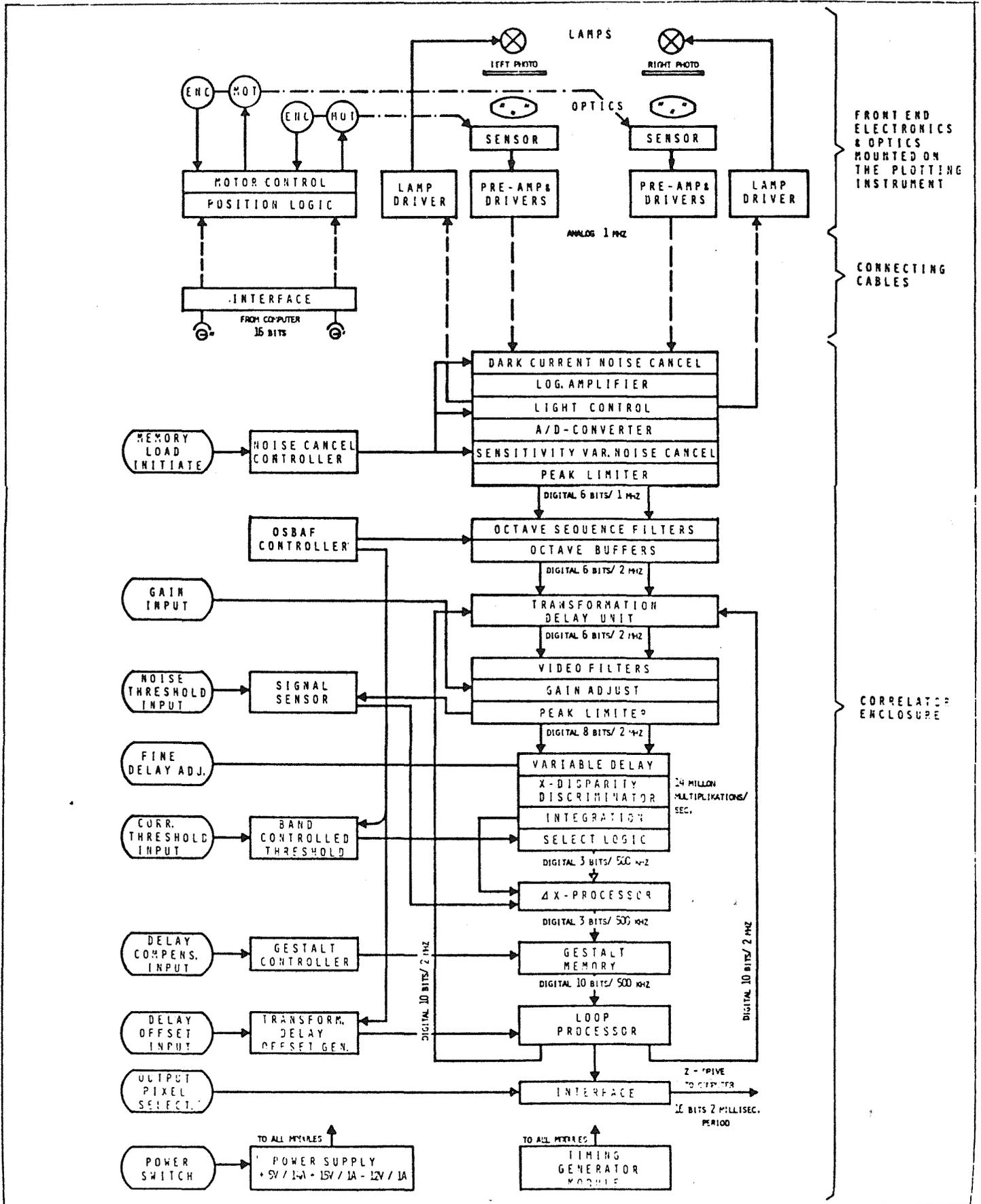
Fig.6: Block Diagram of the Rastar Correlator
