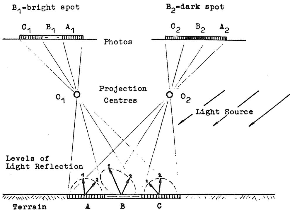
Fig.2: Photometric distortion by different reflection in different viewing angles.
