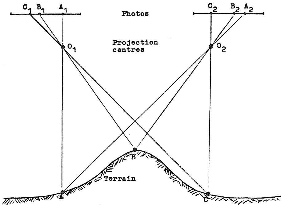
Fig.1: Geometric distortion by terrain elevations
