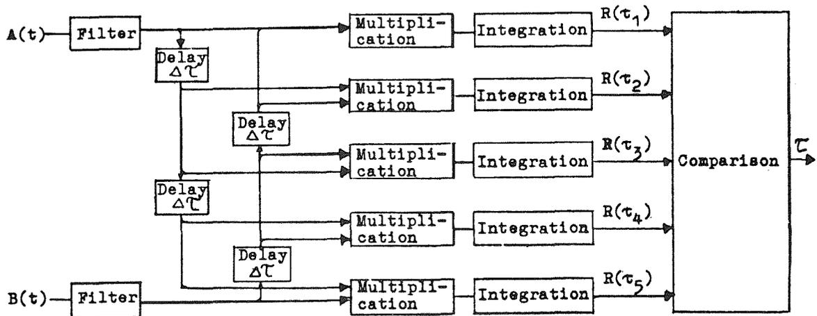
Fig.3: Establishing parallax from maximum correlation function
