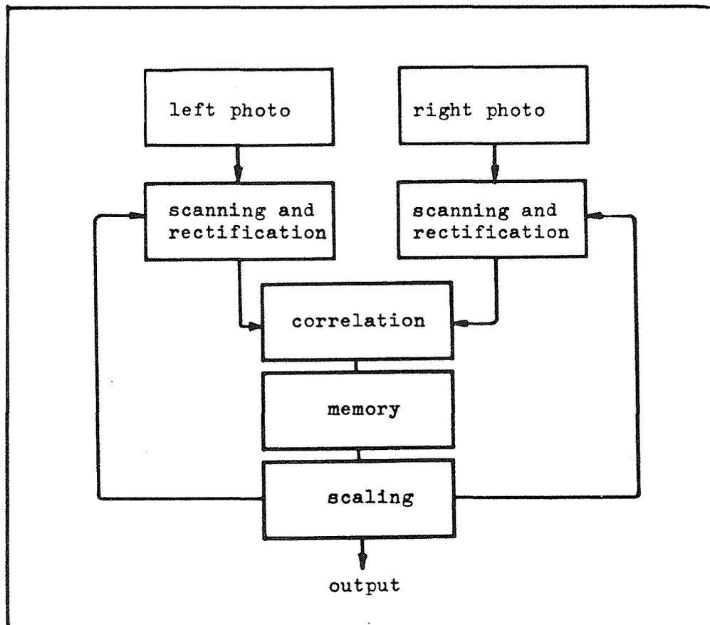
Fig.5: Principle of a correlator with electronic rectification
