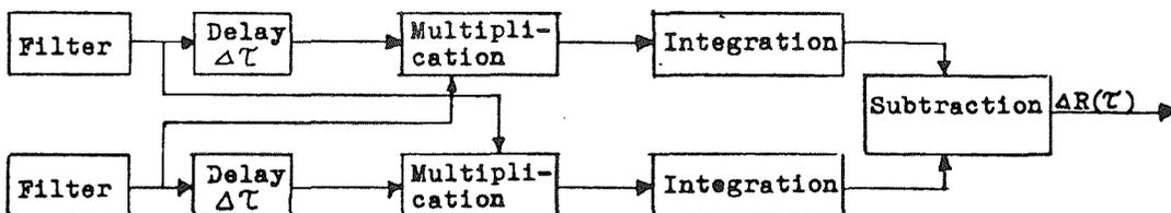
Fig.4: Establishing slope of correlation function for subsequent parallax elimination
