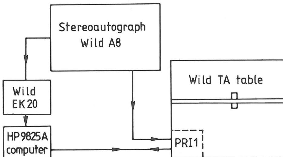
Figure 1. Hardware components of the DOSP-system
