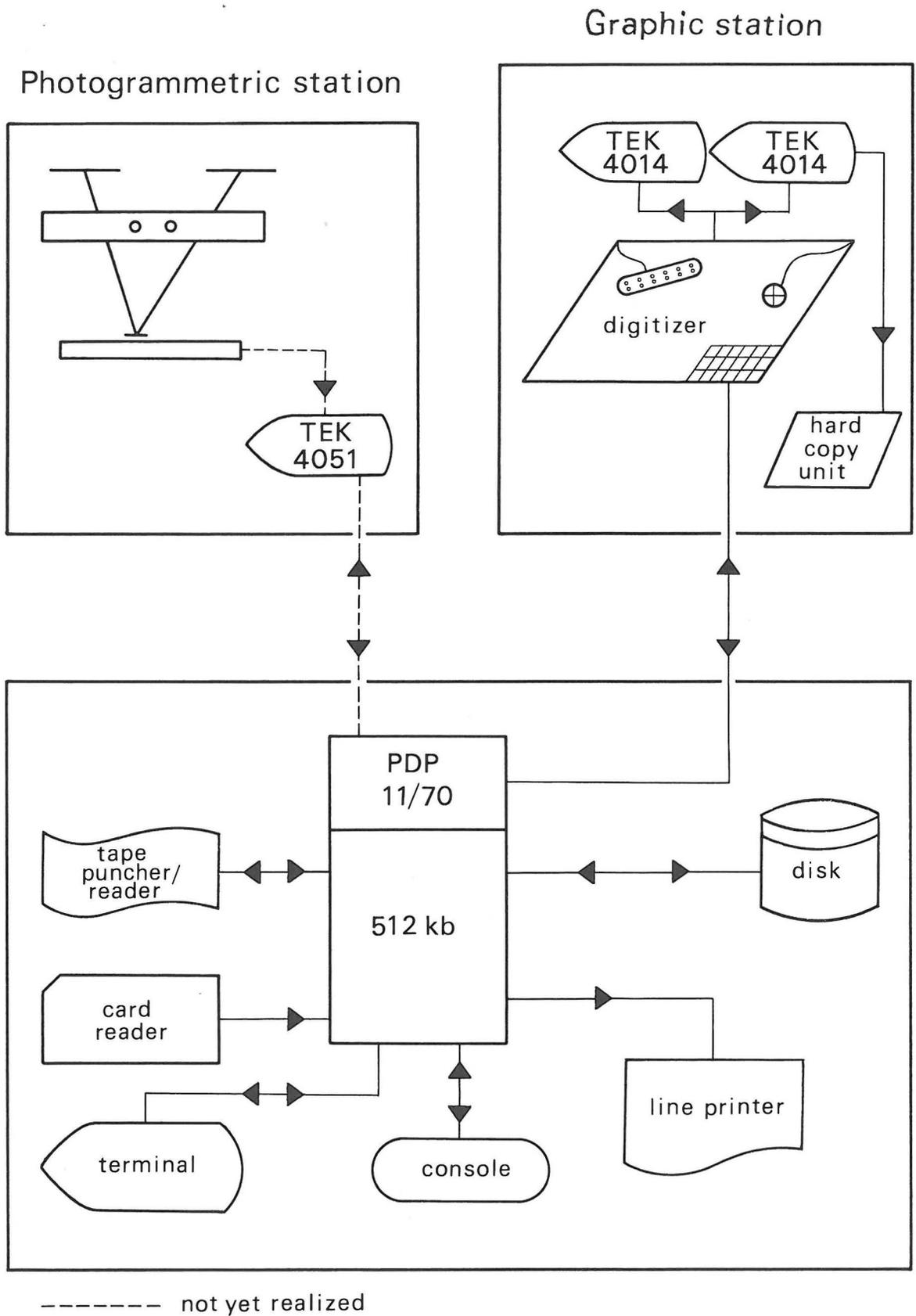
Figure 1: The on-line graphic and photogrammetric station
