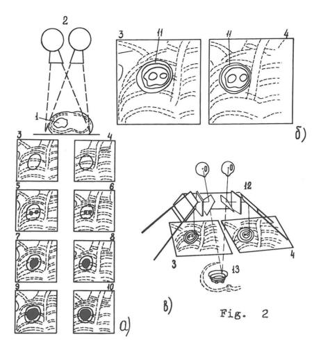
As a result, the first stereopair gives the image of the cavity in horizontals 11 / Fig. 2b /. When this stereopair observed under the stereoscope 12, a protuberance of the cavity wall and the pecularities of its topography are seen in relief / Fig. 2b /.
