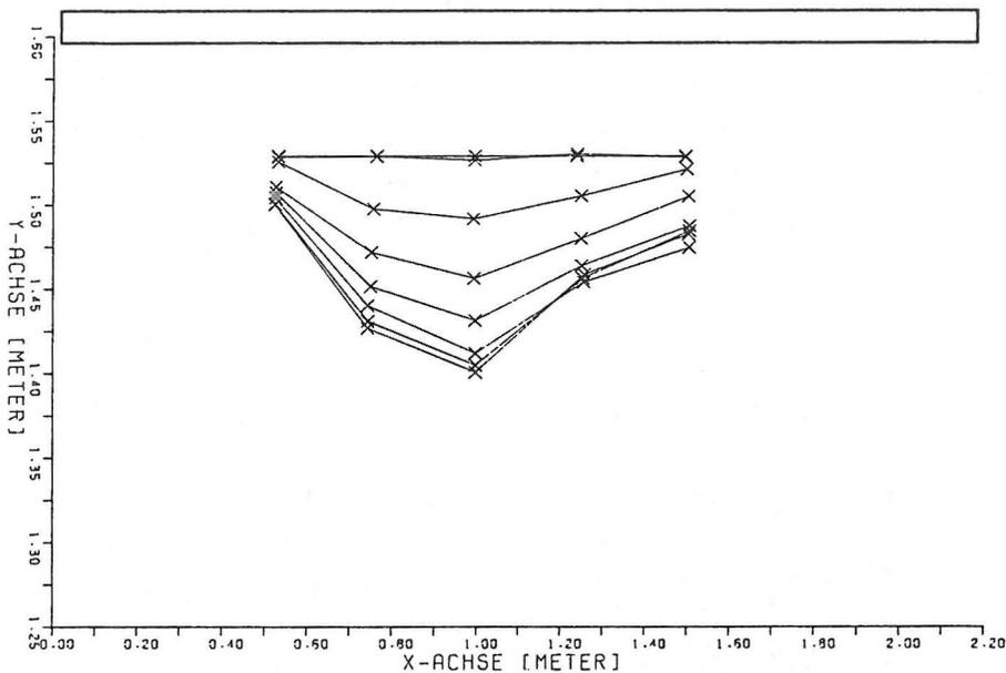
Fig. 4: Deformation of a steel concrete plate in the X-Y-plane at eight equidistant moments  $t$  with  $\Delta t = 0.0025$  seconds, comp. profile 14, Fig. 1 b
