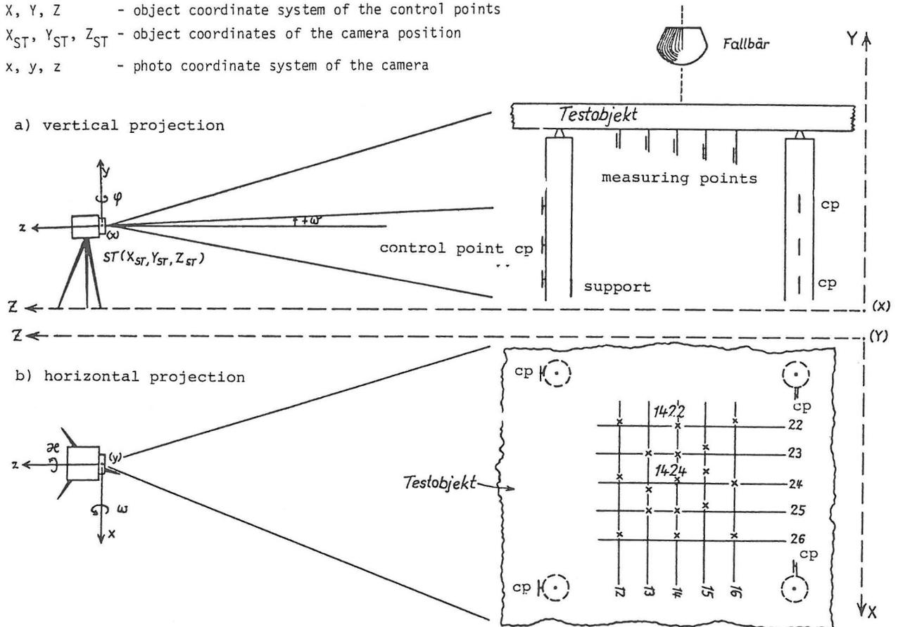
Departing from the consideration that the deformation will occur inside the level stretched by four supports, the test area was marked with a screen of black and white signals. A mutual covering of the marks in the picture must be avoided. This was obtained by fixing the marks on small stalks under the plate; besides they vary in their vertical (fig. 1 a) as well as in the horizontal (fig. 1 b) arrangement.
