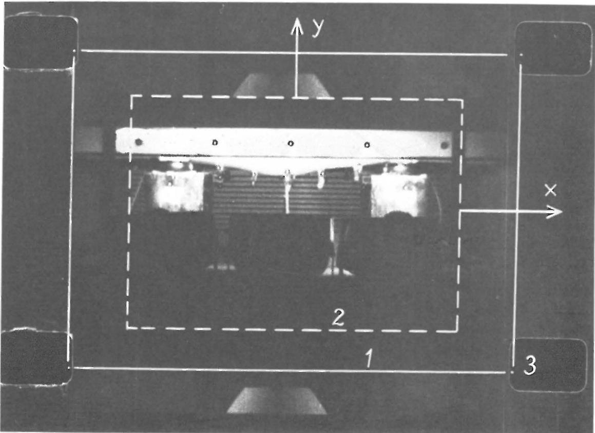
Fig. 3.: Steel concrete plate in the "falling bear" experiment at the moment of maximum deformation (enlargement of a picture with supplements in white)
