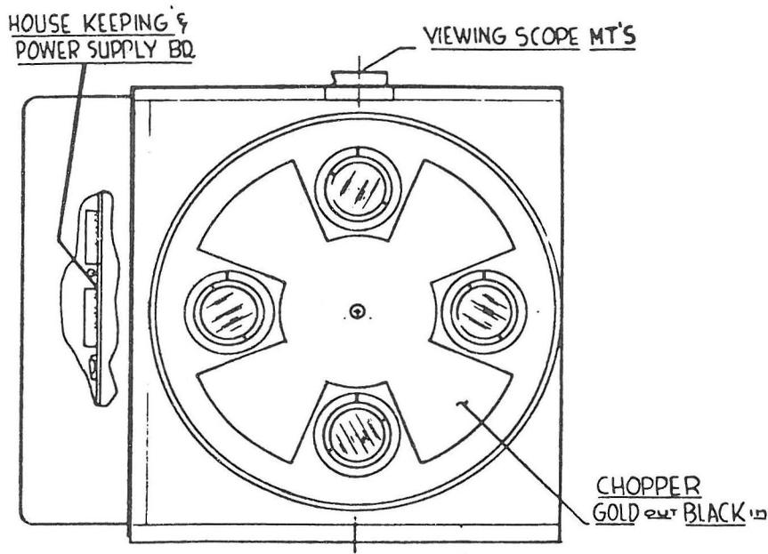
Figure 8. Chopping arrangement for the multiband radiometer.
