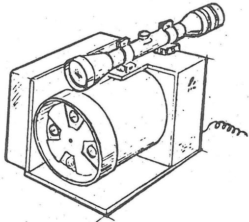
To achieve reliability in reflectance measurement, a field calibration procedure using a reference surface is to be employed for the reflective spectral bands.<sup>10</sup> For the thermal channel, direct field comparison with two reference blackbodies at known temperature will be used to establish the thermal radiance scale.
