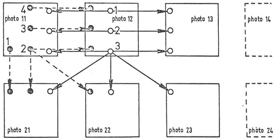
Fig. 2: Systematic procedure of point-transfer and point-marking
