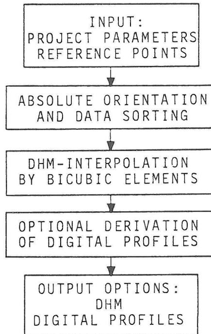
Fig. 4 Block diagram of the program version HIFI-P
