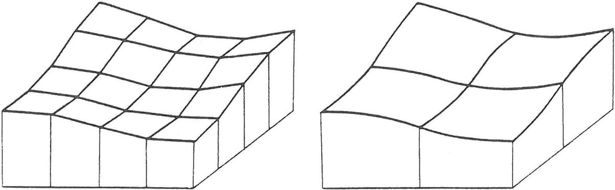
Fig. 3 Interpolation surfaces built respectively of bilinear (left) and bicubic (right) finite elements
