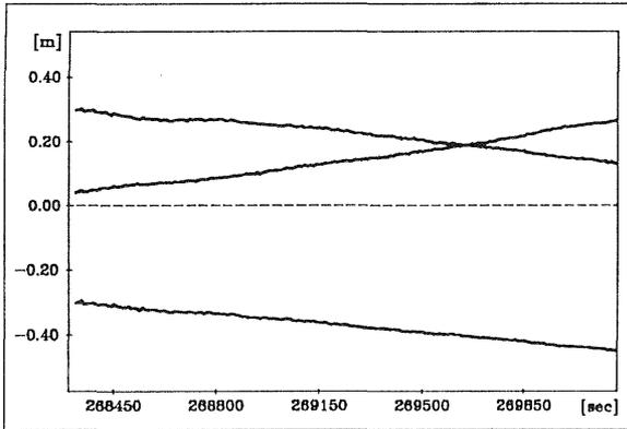
Fig. 1 Systematic Error Effects Due to Incorrect Ambiguities
