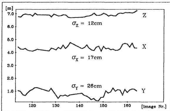
Fig. 5 Coordinate Differences between aerial triangulation and ambiguity resolution algorithm
