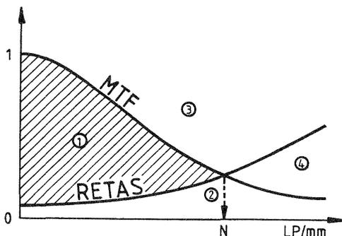
Fig. 2: Pixel size  $N/2$  as a function of MTF and Resolving Threshold of Application System (RETAS). For the numbers see text.
