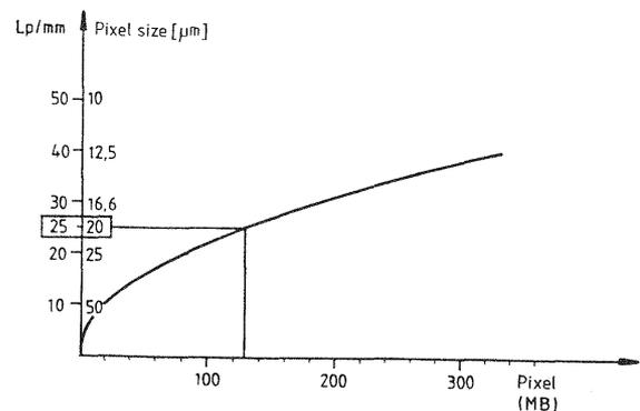
Fig. 1 Data quantity in [MB] as a function of resolution and pixel size for photogrammetric imagery (BÄHR 1989)
