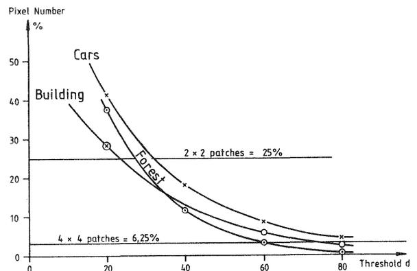
Fig. 8 Reduction of pixel numbers in % as a function of density differences (threshold  $d$ ) and uniform pixel clustering (2 x 2 and 4 x 4 patches)
